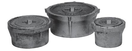
The Model W watertight flush fill caps screw onto the threaded end of fill and/ or sounding lines to provide full diameter access to the tank through a watertight terminal. The assembly consists of a rust-resistant, galvanized cast iron body, with a gasket sealed solid bronze cover for a waterproof seal.
